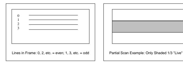
The M30 offers full vertical scanning (normal mode), 1/2 and 1/3 vertical scans. The illustration above shows the middle third of an image being scanned, as indicated by the shaded area. Note that only the shaded area is "live" in this mode, so the area to be measured must appear in this portion. However, this allows some things to be measured with very high time resolution.
