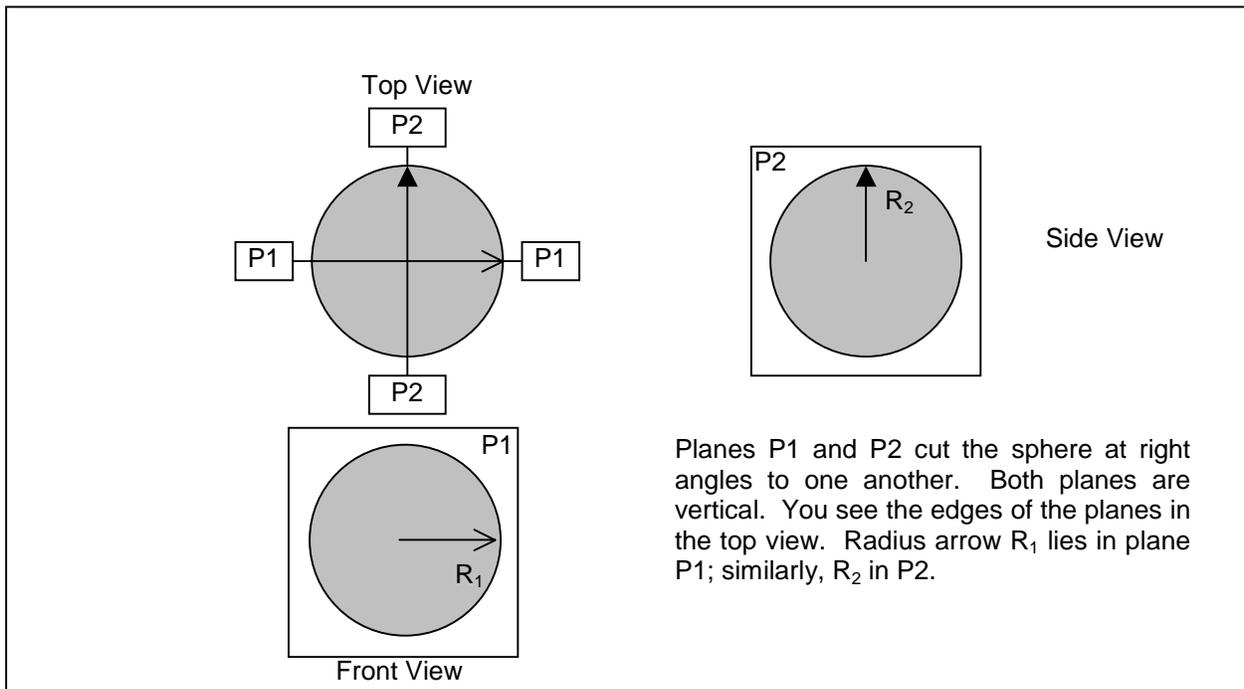
The first important concept is that of radius of curvature: this says that if a sphere were fitted to the surface at a point, then the radius of the sphere is the radius of curvature for that point on the surface. For the spherical drop, this is trivial: the radius of curvature is the radius of the sphere, but for more complex surfaces finding the radius of curvature is difficult.
