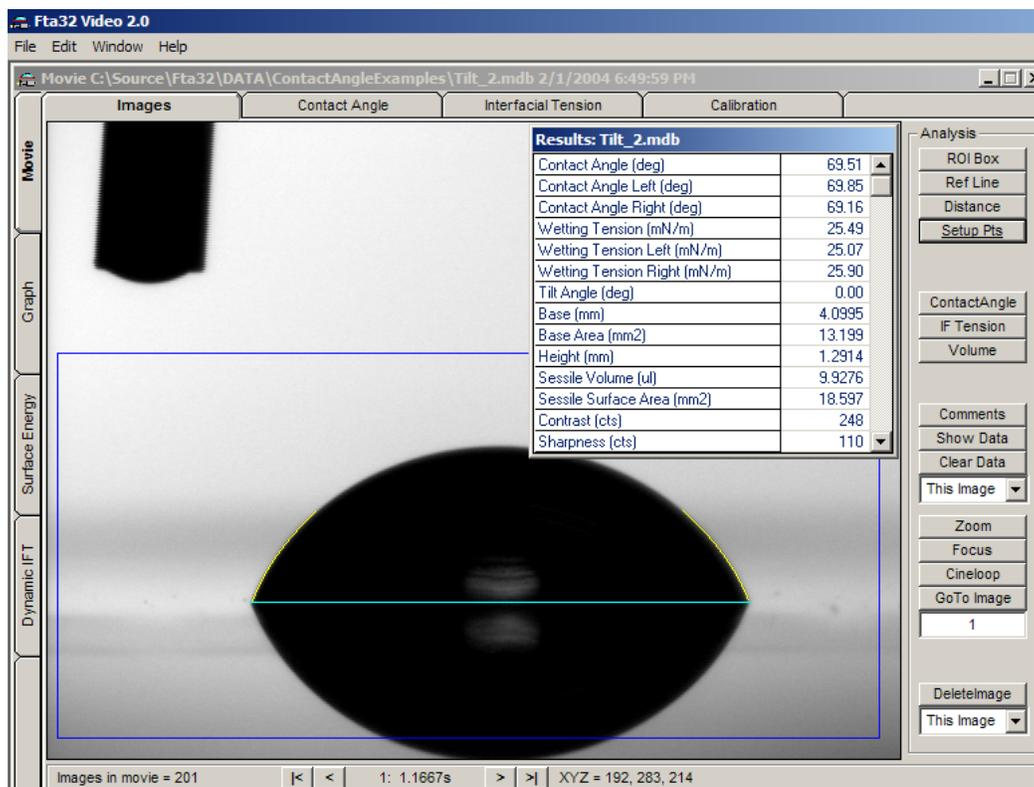
Just starting to tilt. On this FTA2000, the dispense needle does not tilt so it moves out of the image as the table starts. The drop appears level in the image. The ROI box prevents the analysis from considering the dispense needle as an indicator of where the drop is located horizontally.
